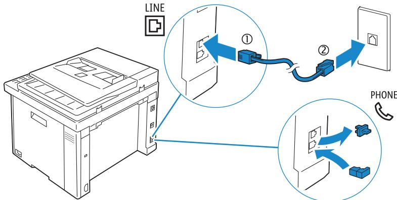
**NOTE:** If the phone communication is serial in your country (such as Germany, Sweden, Denmark, Austria, Belgium, Italy, France and Switzerland), and you are supplied with a yellow terminator, insert the yellow terminator into the phone connector.
